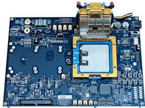
This image shows the optically connected FPGA board developed by Intel and Ayar Labs.
